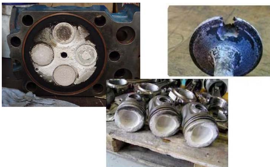
Fig. 1. Defects on engine parts caused by siloxanes [6].
